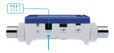
Actuation of the RS-232 port takes place via a special RS-232 cable. If the device shall be actuated via the RS-232 interface, your dealer will be pleased to provide you with a detailed protocol.
